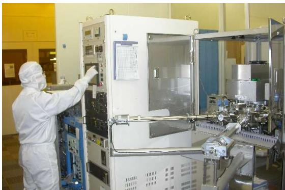
◆ Magnetron RIE system for Al
