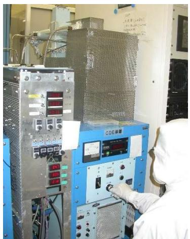
◆ Plasma ashing system for removing
