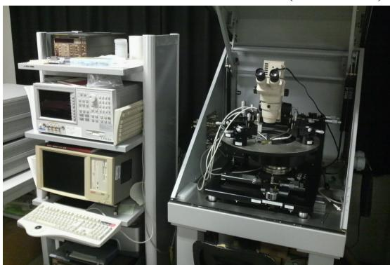
◆ Semi-automatic wafer prober
