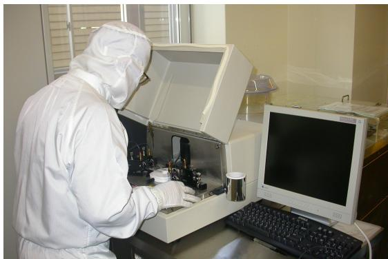
◆ Spectroscopic ellipsometer
