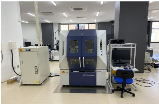
◆ Scanning X-ray photoelectron spectrometer
